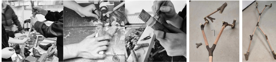
Fig. 8 The design and manufacturing experiment process of translating traditional mortise and tenon structures
