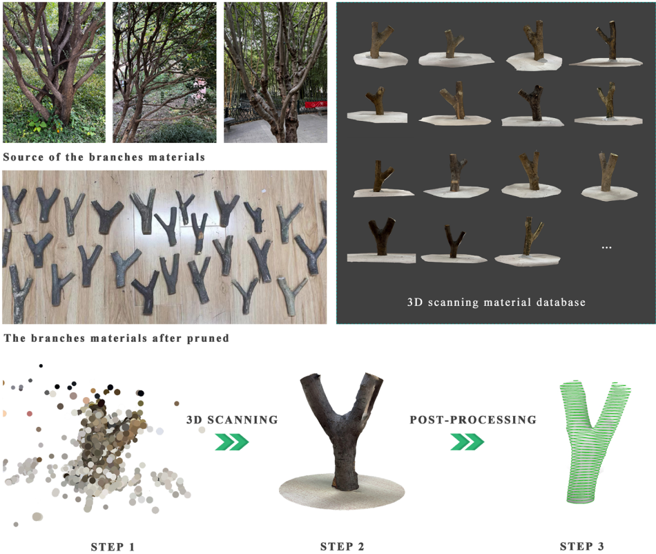
Fig. 2 Data conversion issues in existing material libraries (Including the whole process from material collection to 3D scanning)
